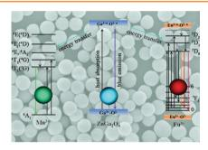
Mn<sub>2+</sub>/Eu<sub>3+</sub> with uniform ZnGa<sub>2</sub>O<sub>4</sub>: morphology nanospheric (diameter about 400 nm) are synthesized via a facile hydrothermal approach. The electronic properties, chemical bonding, and mechanisms of electron transitions in ZnGa<sub>2</sub>O<sub>4</sub> and Mn<sup>2+</sup>/Eu<sup>3+</sup>-doped ZnGa<sub>2</sub>O<sub>4</sub> systems are studied based on the density functional theory (DFT) calculations from first principles.
