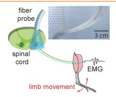
Flexible polymer fiber probes that integrate optical waveguides and conductive electrodes and maintain their functions under dynamic strain are developed. These probes allow simultaneous optogenetic stimulation and recording of neural activity in the spinal cord, which is accompanied by induced limb movements in vivo.
