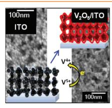
Nanostructured pseudocapacitors are created by coating a conductive scaffold, made through solution-phase templating of ITO nanocrystals, with a conformal layer of vanadium oxide. The materials combine intrinsic electrical conductivity, porosity for solvent diffusion, and short solid-state Li+ diffusion distance. By tuning the vanadia thickness, redox reactions are dominantly pseudocapacitive for vanadia layers up to 7 nm thickness.
