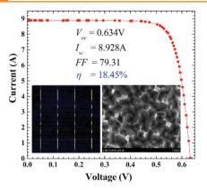
18.45% efficient multi-crystalline silicon solar cells with nanoscale pseudopyramidal texture are fabricated by using a metal-catalyzed chemical etching plus a post alkaline etching. The improved efficiency is mainly ascribed to its enhanced light absorption and acceptable passivation quality, that is, the short-circuit current density has an increase of ≈300 mA cm<sup>-2</sup>, while the open-circuit voltage has only a slight decrease of ≈1 mV.
