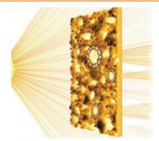
Calcium:silver blend electrodes show extraordinarily high mean transmittance of 93.0% in the visible spectral range, low sheet resistance of 27.3  $\Omega/\Box$ , and excellent flexibility, superior to commonly used indium tin oxide. The unique microstructure enables broadband transmittance enhancement due to plasmonic coupling. Top-illuminated OPV cells using such metal blends as top electrode achieve an outstanding power conversion efficiency of 7.2%.
